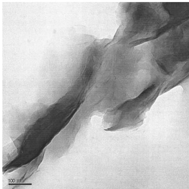
Figure 6 Micrograph of the MAPP/MMT5 nanocomposite.
